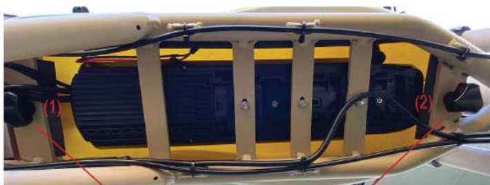
Tank cover retaining fasteners
